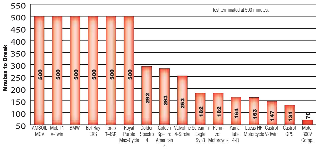
The test shows that 50% of the SAE 40 group oils and only 37.5% of the SAE 50 group oils achieved the maximum obtainable results of 500 minutes. The results of the remaining oils suggest a faster rate of degradation and shorter service life.
