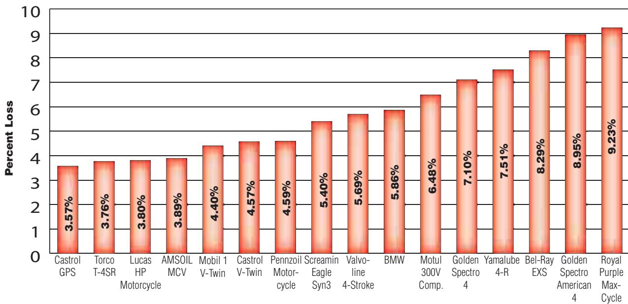
The results show a significant difference between those oils with low volatility and those with higher volatility. Low volatility is of particular benefit in hot running, air-cooled engines.
