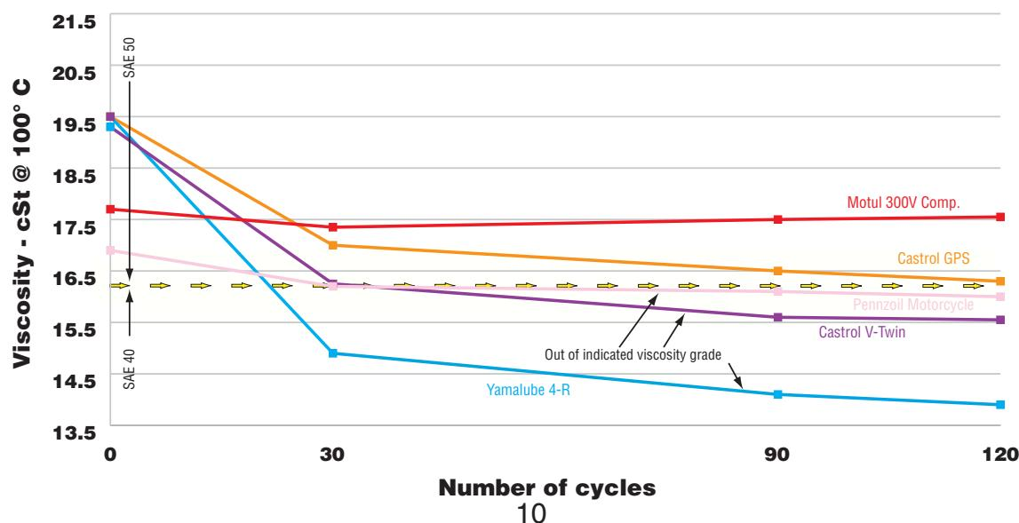
The results point out significant differences between oils and their ability to retain their viscosity. Within the SAE 40 group, 41.6% of the oils dropped one viscosity grade to an SAE 30. Within the SAE 50 group, 43.8% dropped one grade to an SAE 40. Most of the oils losing a viscosity grade did so quickly, within the initial 30 cycles of shearing. Testing revealed that Lucas 10W-40 High Performance Motorcycle oil was the only oil to shear to an SAE 20.
